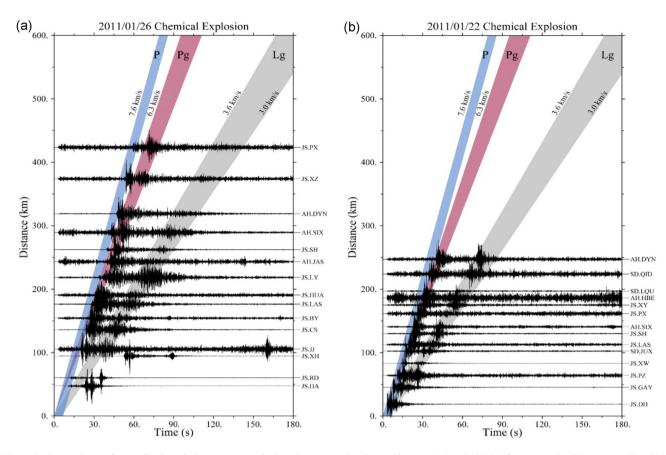
**Figure 3.** Comparisons of normalized vertical-component velocity seismograms bandpassed between 5.0 and 10.0 Hz for two nearby CExs occurred on 2011 January 26 (a) and 22 (b). The horizontal and vertical coordinates are time and epicentre distance. The *P*, Pg and Lg group velocities are indicated by shaded strips. Note that the waveforms show common features of clear impulsive *P*-wave onset and relatively weak Lg phases.
