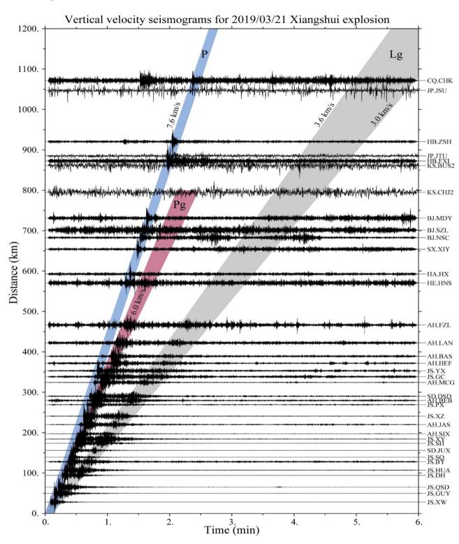
Figure 2. Normalized vertical-component velocity seismograms bandpass filtered between 5.0 and 10.0 Hz for the 2019 March 21 XEx. The traces are ordered according to their epicentral distances, with station names listed on the right side. The three shaded strips indicate *P*, Pg and Lg group velocity windows, respectively.
