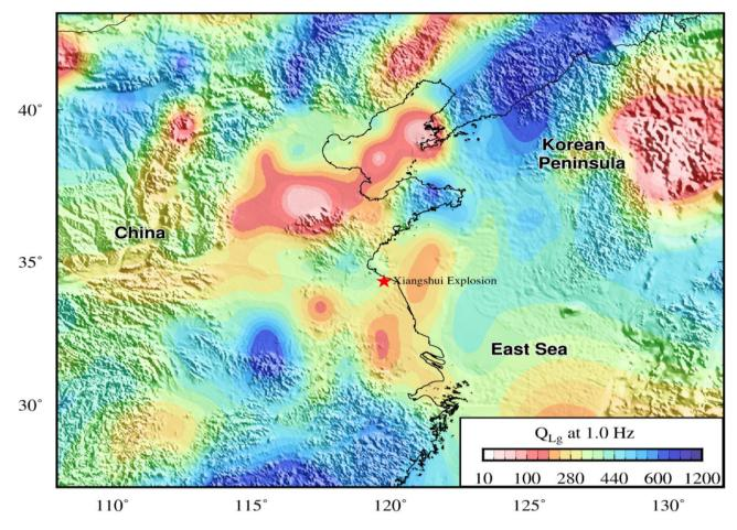
Figure 6. Crustal Lg wave Q map at 1.0 Hz for the investigated region (Zhao et al. 2013).
