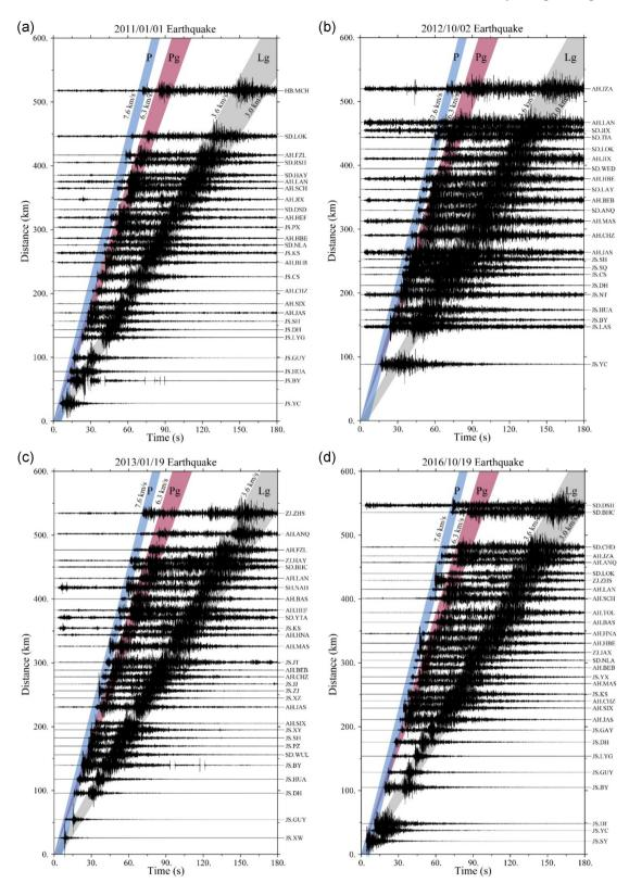
Figure 4. Similar to Fig. 3 except for four nearby earthquakes occurred on 2011 January 1 (a), 2011 October 2 (b), 2013 January 19 (c) and 2016 October 19 (d) recorded by stations listed on the right side. The waveforms are characterized by well-developed Lg phases.
