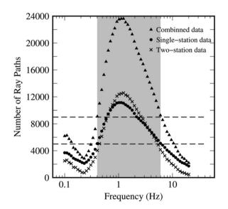
Fig.4 The numbers of available rays, including both single-station and two-station rays, at individual frequencies from 0.1 to 20.0 Hz. The shaded area highlights the 0.4–6.0 Hz band, within which the resolution can reach to ~  $1.0^{\circ} \times 1.0^{\circ}$
